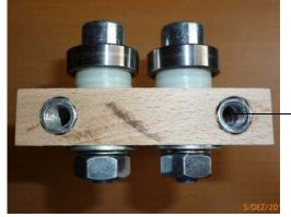
Here you can see how the screw sleeves are pressed into the holes.
