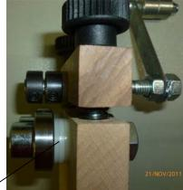
Detailled view on the "action side". You can see the 3 polyamid washers adjusting the ball bearings to sit in the middle of the 2 drillstops.
