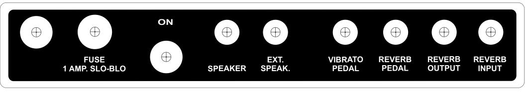
This is the front- and back panel in 1:1 scale, which can also be used as a drill template.
