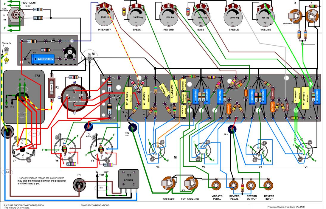
REMARK: FORM A SLOPE SO THAT PE-CONNECTION WILL BECOME THE LAST TO STRIP OFF IN CASE OF PULLING FORCE TO MAINS CABLE:
